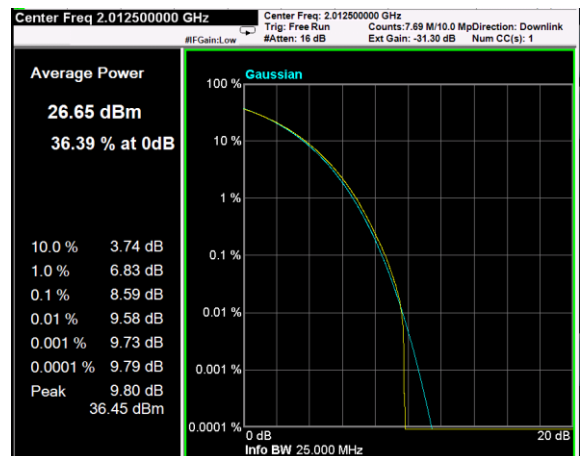
Channel: TOP, Modulation: 16QAM, BW=15MHz, CCDF
