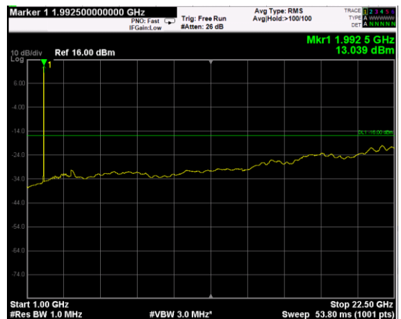
Channel: TOP, Modulation: 64QAM, BW=5MHz, Range: Upper
