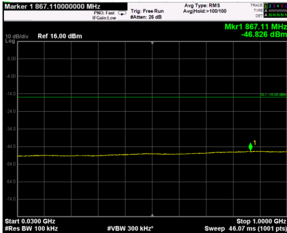
Channel: MIDDLE, Modulation: QPSK, BW=20MHz, Range: Lower
