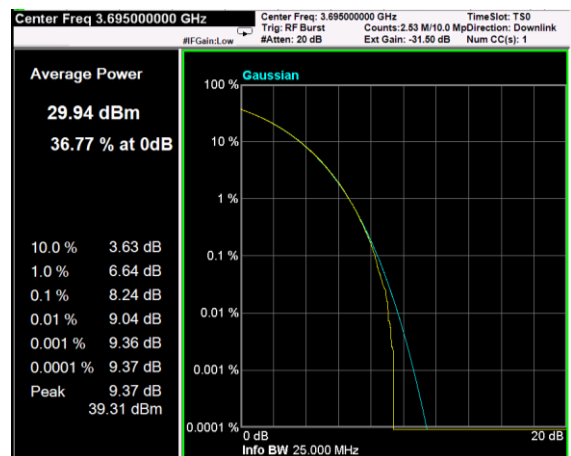
Channel: TOP, Modulation: 64QAM, BW=10MHz, CCDF
