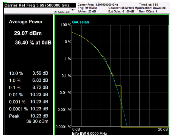
Channel: TOP, Modulation: 256QAM, BW=5MHz, CCDF
