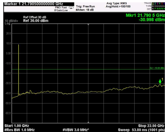
Channel: MIDDLE, Modulation: 16QAM, BW=15MHz, Range: Upper
