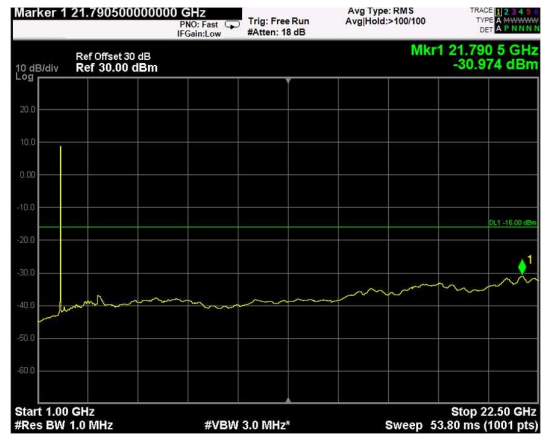
Channel: MIDDLE, Modulation: 64QAM, BW=20MHz, Range: Upper
