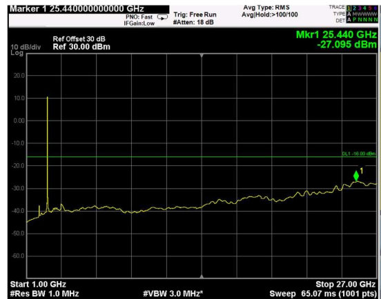
Channel: MIDDLE, Modulation: 256QAM, BW=10MHz, Range: Upper
