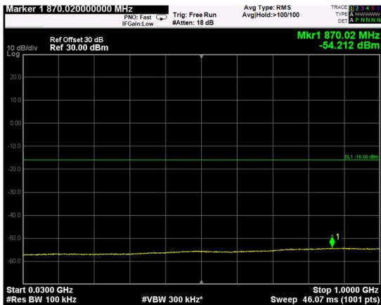
Channel: MIDDLE, Modulation: 256QAM, BW=5MHz, Range: Lower
