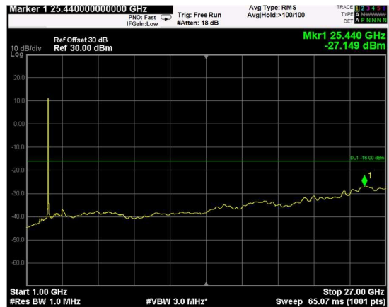
Channel: MIDDLE, Modulation: 16QAM, BW=15MHz, Range: Upper
