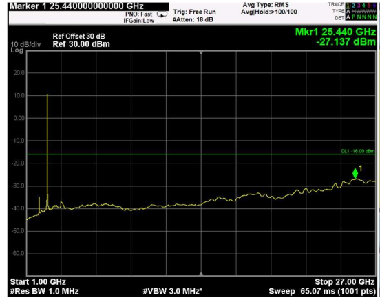
Channel: BOTTOM, Modulation: 64QAM, BW=10MHz, Range: Upper
