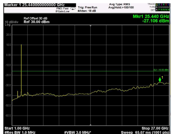
Channel: TOP, Modulation: 16QAM, BW=10MHz, Range: Upper
