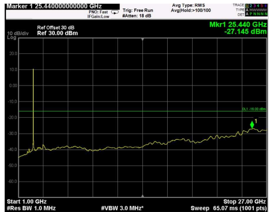
Channel: MIDDLE, Modulation: 64QAM, BW=15MHz, Range: Upper
