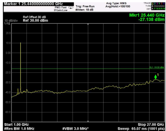
Channel: MIDDLE, Modulation: 256QAM, BW=15MHz, Range: Upper
