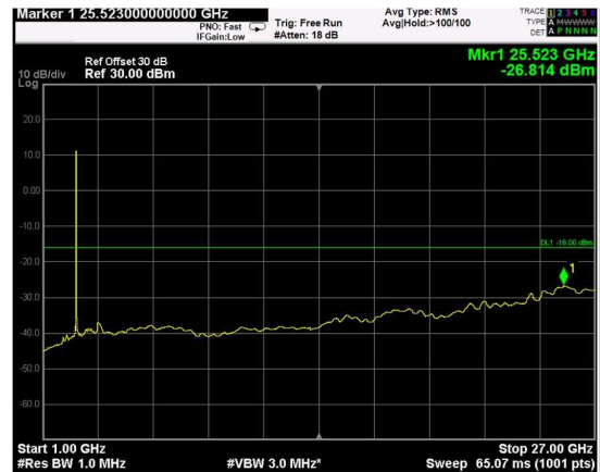
Channel: MIDDLE, Modulation: 16QAM, BW=5MHz, Range: Upper
