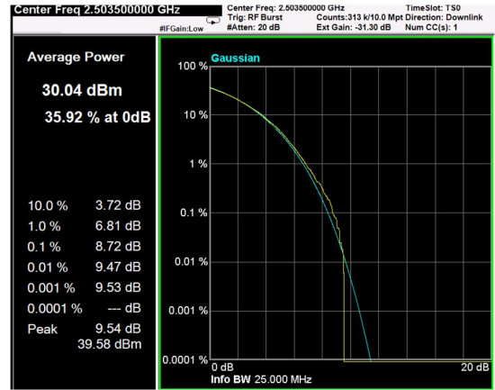
Channel: BOTTOM, Modulation: 64QAM, BW=15MHz, CCDF
