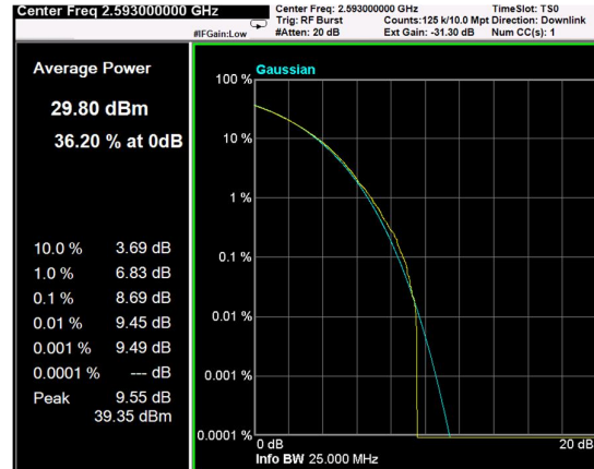
Channel: MIDDLE, Modulation: QPSK, BW=15MHz, CCDF
