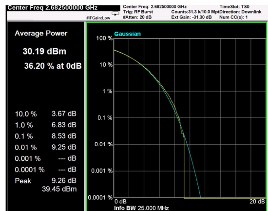
Channel: TOP, Modulation: 64QAM, BW=15MHz, CCDF
