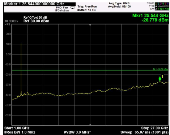
Channel: MIDDLE, Modulation: QPSK, BW=5MHz, Range: Upper
