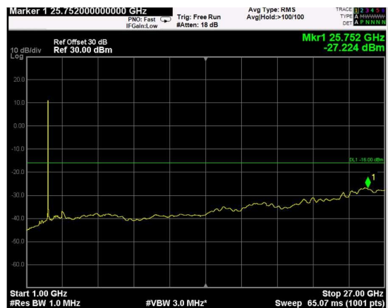
Channel: TOP, Modulation: 64QAM, BW=5MHz, Range: Upper
