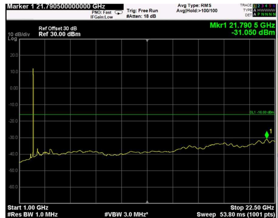
Channel: MIDDLE, Modulation: 256QAM, BW=5MHz, Range: Upper
