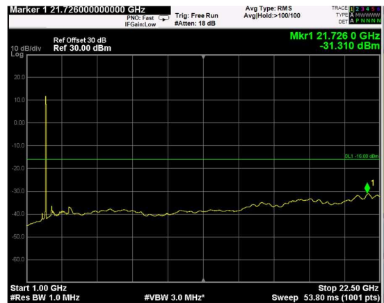
Channel: TOP, Modulation: QPSK, BW=15MHz, Range: Upper
