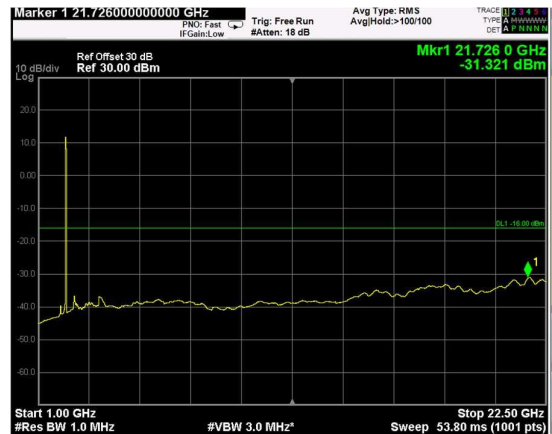
Channel: MIDDLE, Modulation: 16QAM, BW=15MHz, Range: Upper
