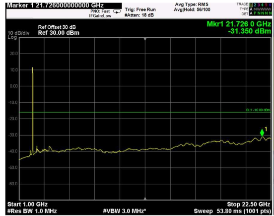
Channel: BOTTOM, Modulation: 256QAM, BW=15MHz, Range: Upper
