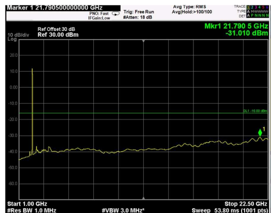
Channel: TOP, Modulation: 256QAM, BW=5MHz, Range: Upper
