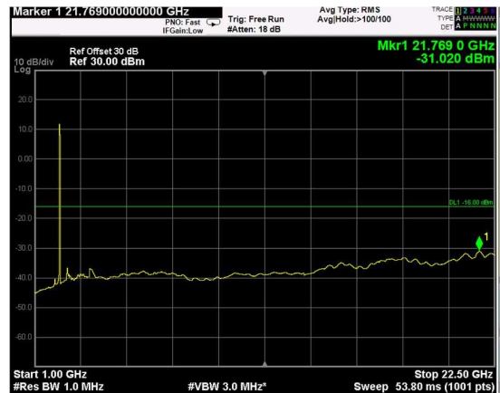
Channel: MIDDLE, Modulation: 16QAM, BW=20MHz, Range: Upper
