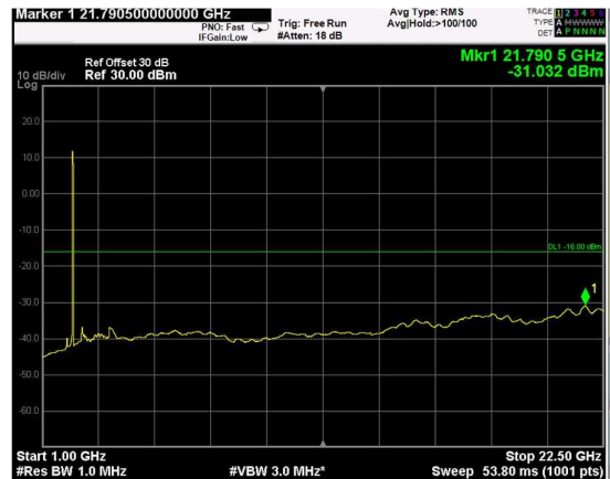
Channel: MIDDLE, Modulation: 64QAM, BW=5MHz, Range: Upper
