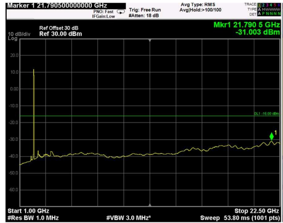
Channel: BOTTOM, Modulation: 256QAM, BW=5MHz, Range: Upper
