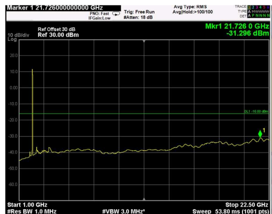
Channel: TOP, Modulation: 16QAM, BW=15MHz, Range: Upper
