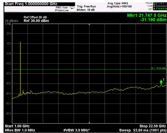
Channel: MIDDLE, Modulation: 64QAM, BW=10MHz, Range: Upper
