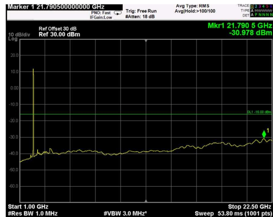
Channel: TOP, Modulation: 16QAM, BW=15MHz, Range: Upper
