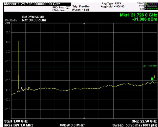
Channel: TOP, Modulation: 64QAM, BW=5MHz, Range: Upper
