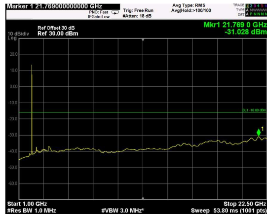
Channel: MIDDLE, Modulation: 16QAM, BW=15MHz, Range: Upper
