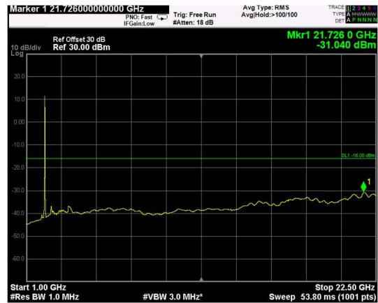
Channel: MIDDLE, Modulation: 256QAM, BW=5MHz, Range: Upper
