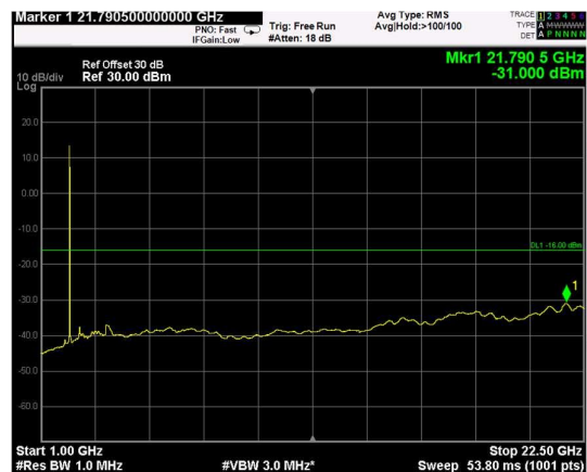
Channel: TOP, Modulation: 256QAM, BW=20MHz, Range: Upper
