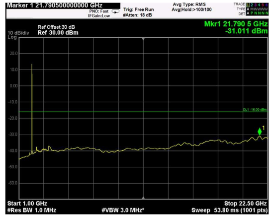
Channel: BOTTOM, Modulation: 16QAM, BW=20MHz, Range: Upper
