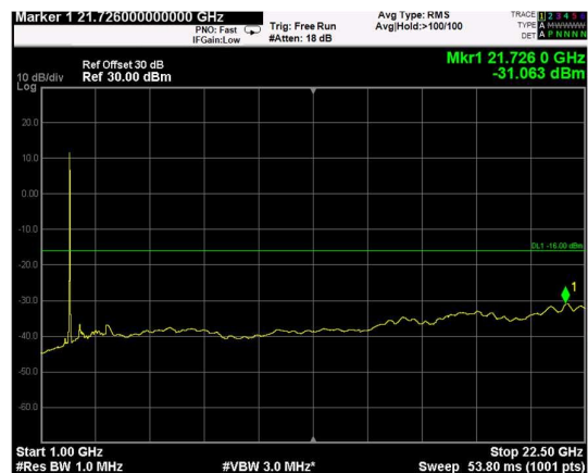
Channel: TOP, Modulation: 256QAM, BW=5MHz, Range: Upper
