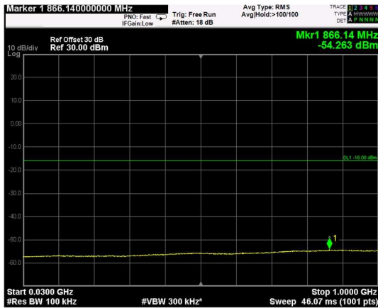
Channel: MIDDLE, Modulation: QPSK, BW=15MHz, Range: Lower
