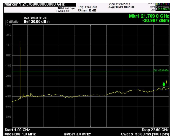
Channel: TOP, Modulation: 256QAM, BW=15MHz, Range: Upper
