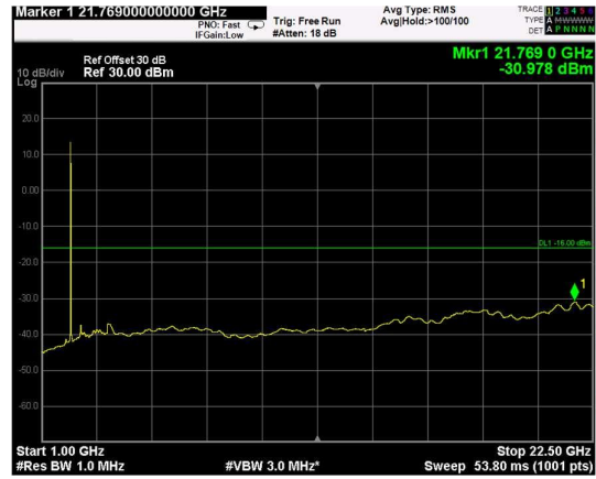
Channel: BOTTOM, Modulation: 256QAM, BW=20MHz, Range: Upper
