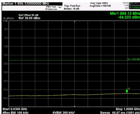
Channel: TOP, Modulation: 16QAM, BW=5MHz, Range: Lower
