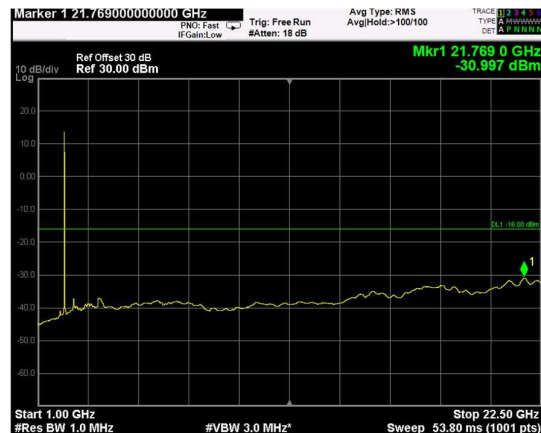
Channel: TOP, Modulation: 16QAM, BW=15MHz, Range: Upper
