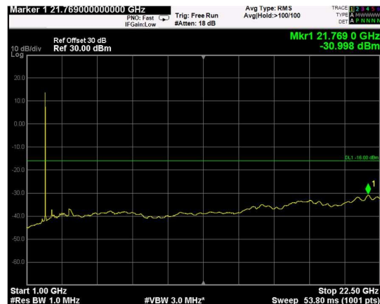
Channel: TOP, Modulation: 16QAM, BW=20MHz, Range: Upper
