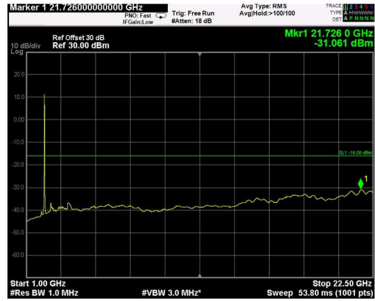
Channel: BOTTOM, Modulation: 64QAM, BW=5MHz, Range: Upper
