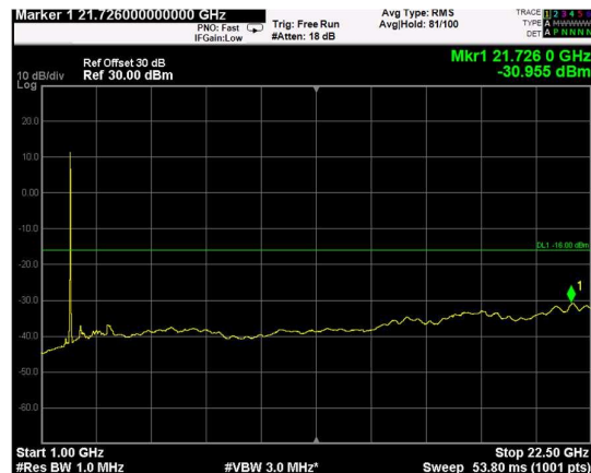
Channel: TOP, Modulation: 16QAM, BW=5MHz, Range: Upper
