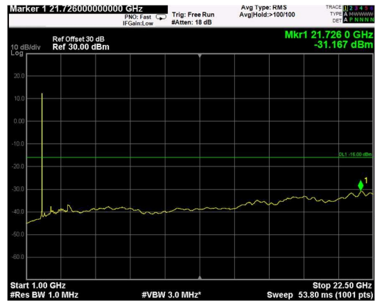
Channel: MIDDLE, Modulation: QPSK, BW=5MHz, Range: Upper
