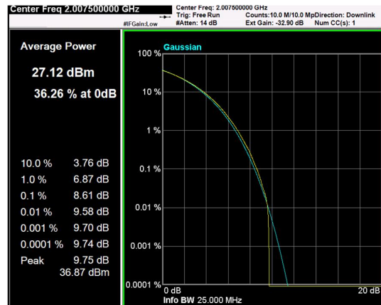
Channel: MIDDLE, Modulation: 256QAM, BW=15MHz, CCDF
