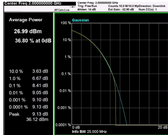
Channel: BOTTOM, Modulation: 16QAM, BW=10MHz, CCDF
