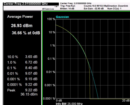
Channel: TOP, Modulation: 64QAM, BW=10MHz, CCDF
