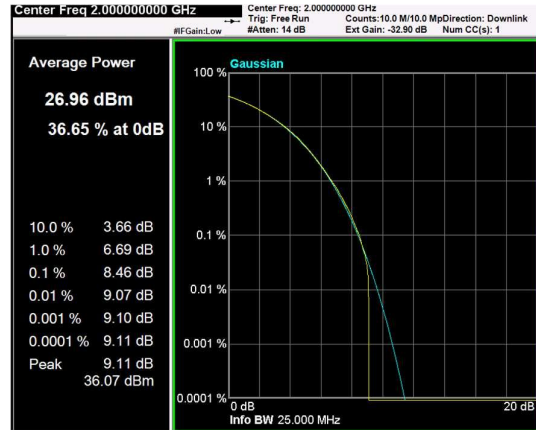
Channel: BOTTOM, Modulation: QPSK, BW=10MHz, CCDF
