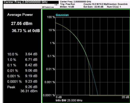
Channel: BOTTOM, Modulation: 64QAM, BW=20MHz, CCDF
