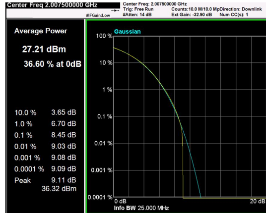
Channel: MIDDLE, Modulation: QPSK, BW=10MHz, CCDF
