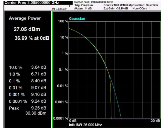
Channel: BOTTOM, Modulation: 16QAM, BW=20MHz, CCDF
