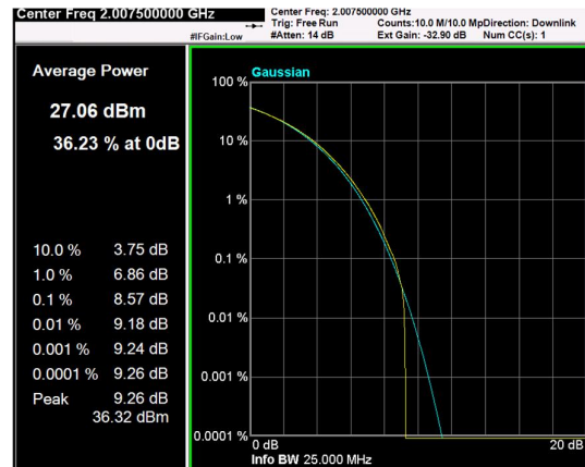
Channel: MIDDLE, Modulation: 256QAM, BW=10MHz, CCDF
