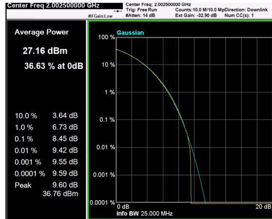
Channel: BOTTOM, Modulation: 256QAM, BW=15MHz, CCDF
