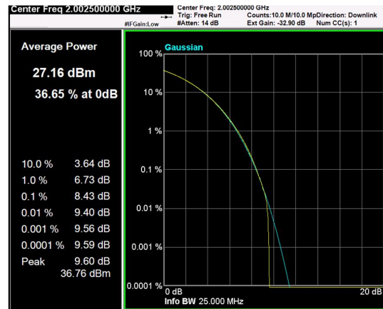
Channel: BOTTOM, Modulation: 16QAM, BW=15MHz, CCDF
