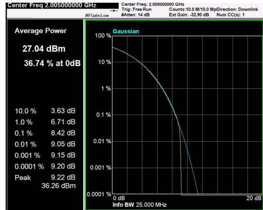
Channel: BOTTOM, Modulation: 256QAM, BW=20MHz, CCDF
