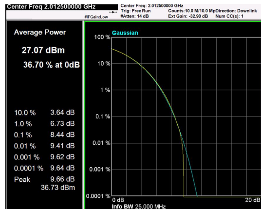
Channel: TOP, Modulation: 64QAM, BW=15MHz, CCDF
