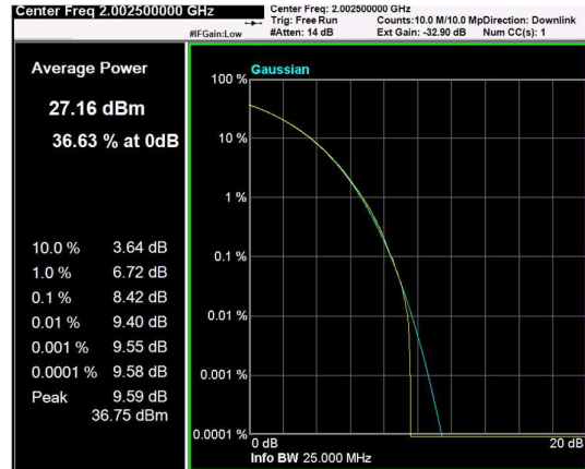
Channel: BOTTOM, Modulation: QPSK, BW=15MHz, CCDF
