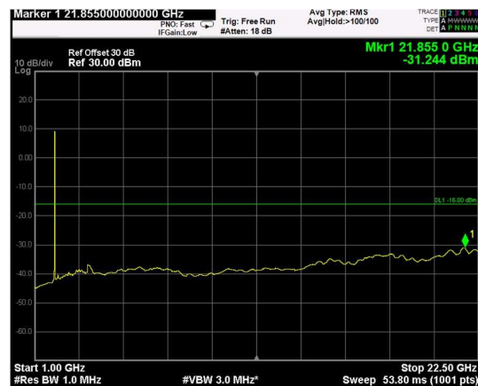
Channel: TOP, Modulation: QPSK, BW=5MHz, Range: Upper
