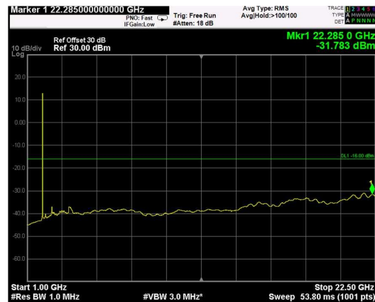
Channel: TOP, Modulation: QPSK, BW=15MHz, Range: Upper
