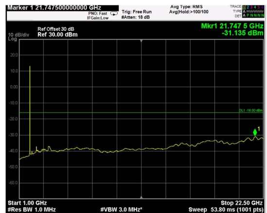
Channel: TOP, Modulation: 16QAM, BW=20MHz, Range: Upper
