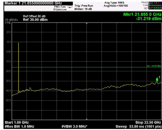
Channel: BOTTOM, Modulation: 64QAM, BW=5MHz, Range: Upper
