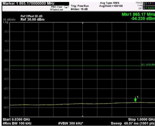
Channel: MIDDLE, Modulation: QPSK, BW=15MHz, Range: Lower
