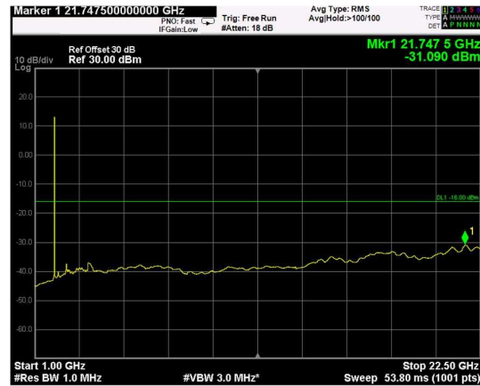
Channel: MIDDLE, Modulation: QPSK, BW=15MHz, Range: Upper
