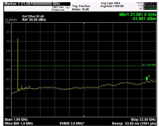
Channel: MIDDLE, Modulation: 64QAM, BW=10MHz, Range: Upper
