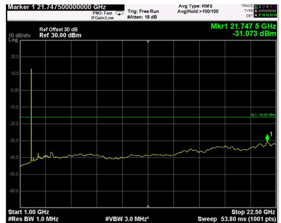
Channel: TOP, Modulation: 64QAM, BW=20MHz, Range: Upper
