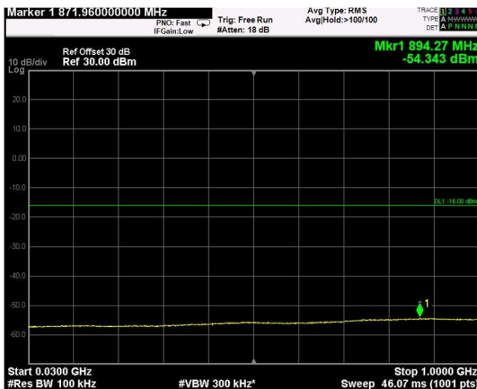
Channel: TOP, Modulation: 256QAM, BW=15MHz, Range: Lower
