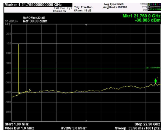
Channel: TOP, Modulation: 64QAM, BW=5MHz, Range: Upper
