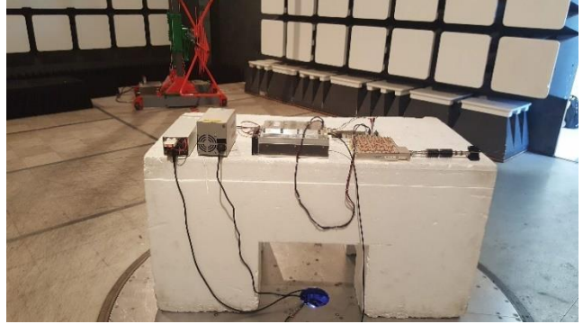
Figure 9.1-2: Radiated setup photo below 1 GHz
