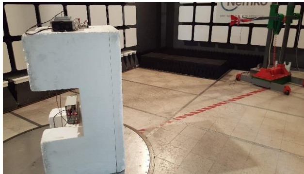
Figure 9.1-3: Radiated setup photo above 1 GHz
