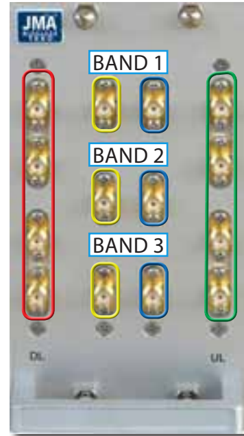
Triplexer with built-in 4-way Combiner/Splitter
