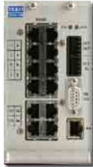
Supervision Module with RS232 connector
