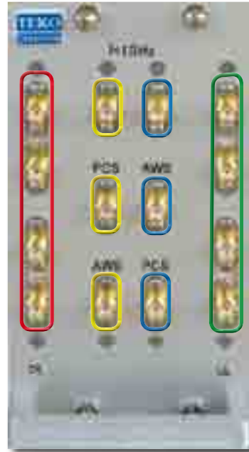
Example: AMPS, PCS, AWS Triplexer with built-in 4-way Combiner/Splitter
