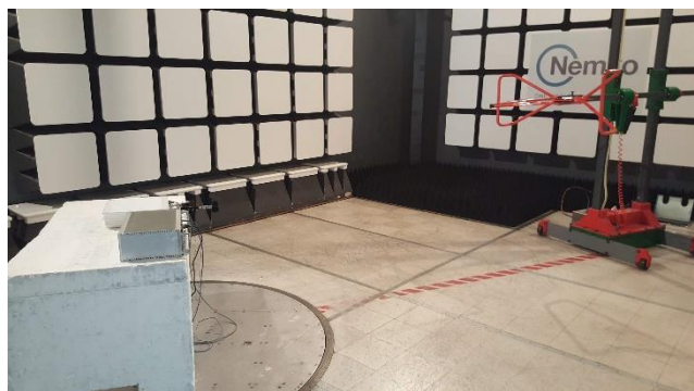
Figure 9.1-1: Radiated setup photo below 1 GHz
