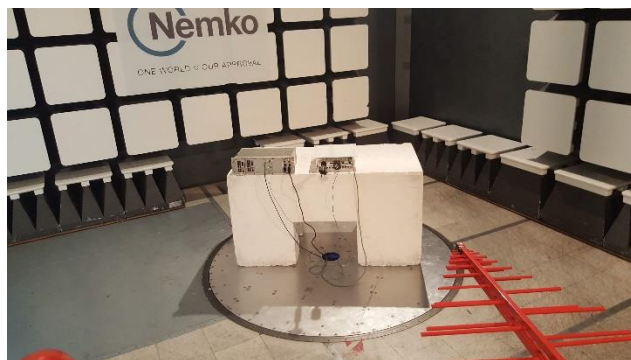
Figure 9.1-2: Radiated setup photo below 1 GHz
