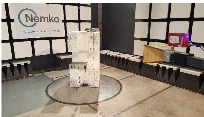
Figure 9.1-4: Radiated setup photo above 1 GHz
