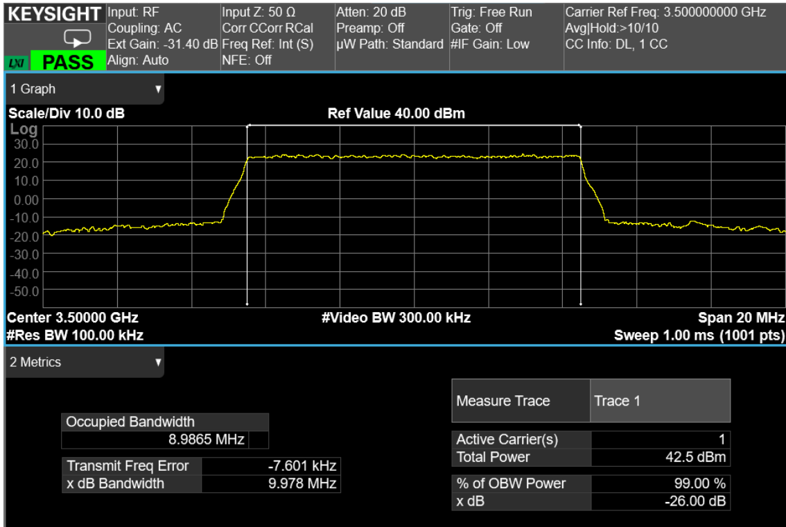
10 MHz signal, middle channel, nominal input signal + 3dB - Output
