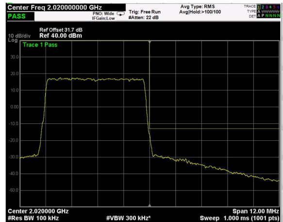
AWGN Signal, Nominal Input Signal +3dB, High Band Edge, 1 Carrier
