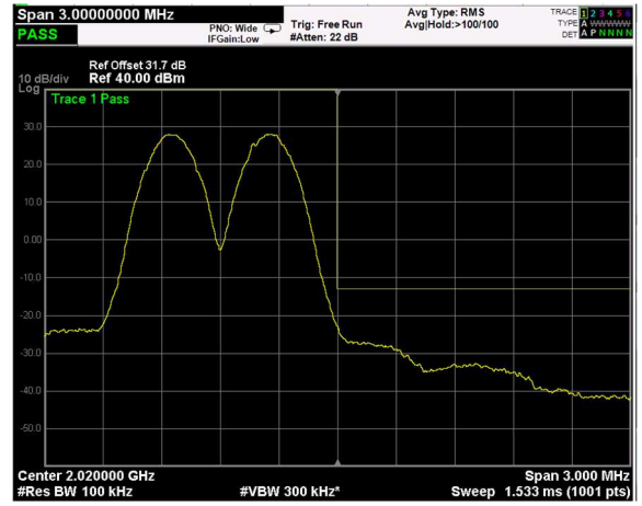
MSK Signal, Nominal Input Signal +3dB, High Band Edge, 2 Carrier
