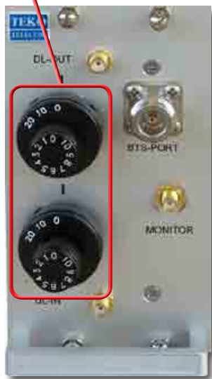
Passive POI with built-in duplexer
