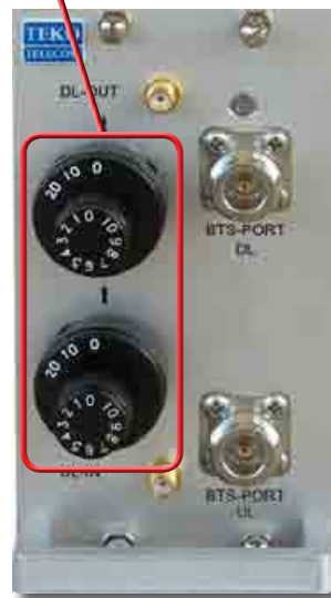
Passive POI without built-in duplexer
