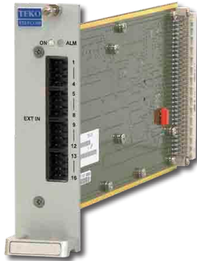
Alarm Board equipped with 16 input pins - TEA-I16
