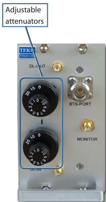
Passive POI with built-in duplexer
