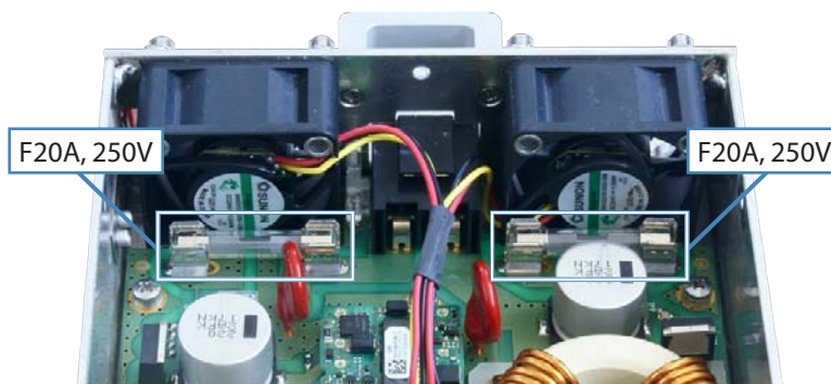
DC/DC Power Supply module (TPSU/48-30-1K) input protection fuses - position and electrical rating
