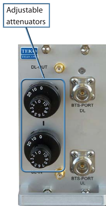
Passive POI without built-in duplexer
