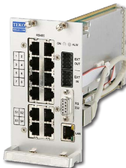
Supervision Module with RS232 port
