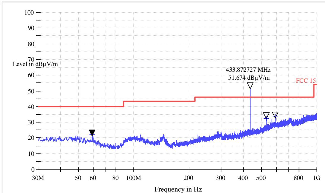
**Remark: The 433.872MHz is the un-modulated CW signal from the SIGNAL Generator**
