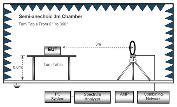
(B) Radiated Emission Test-Up Frequency 30MHz~1GHz
