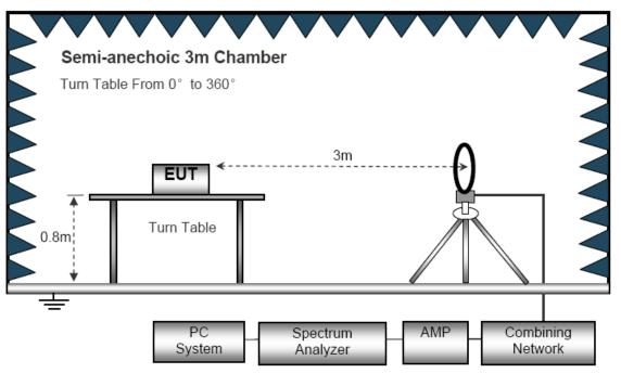
(B) Radiated Emission Test-Up Frequency 30MHz~1GHz
