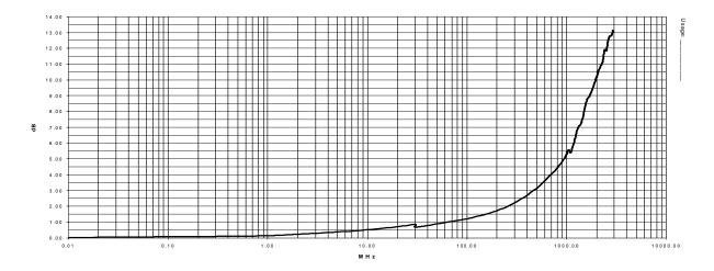
Radiated at 3 meters; 30MHz through 3000MHz, Coax #9812\_11 Last Calibration date: Nov 19, 2008
