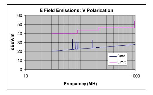
Vertically polarized Class B Graph of Spurious Quasi-Peak Measurements
