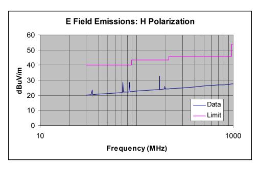
Horizontally Polarized Class B Graph of Spurious Quasi-Peak Measurements
