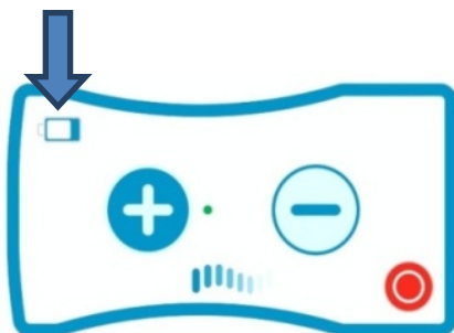
Low Battery Indicator
