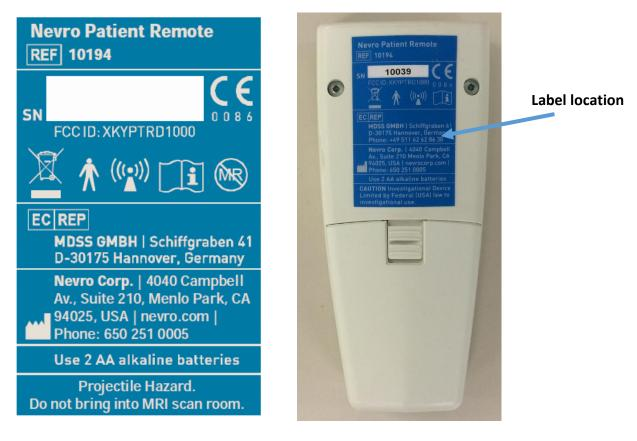
Labels are permanently attached to the device with adhesive and are resistant against wear.
