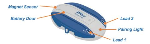
**Remote Control:** The Remote Control (model PTRC3000T) is a handheld, battery-operated unit that communicates with the Trial Stimulator using Bluetooth<sup>®</sup> wireless technology. The patient can use the Remote Control to turn stimulation on or off and adjust certain therapy settings, as well as retrieve the current stimulation level and battery status from the Trial Stimulator.
