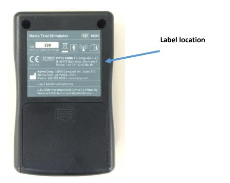
Labels are permanently attached to the device with adhesive and are resistant against wear.
