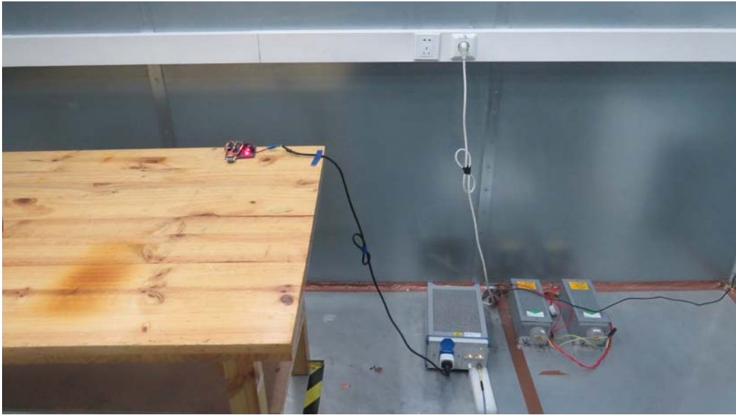
Picture 3 Conducted Emission Test Setup
