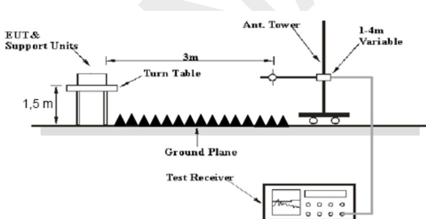
The radiated emission tests were performed in the 3 meters chamber test site, using the setup accordance with the ANSI C63.10-2013. The specification used was the FCC 15.209, and FCC 15.247 limits.
