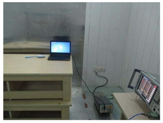
FCC RADIATED EMISSION TEST SETUP
