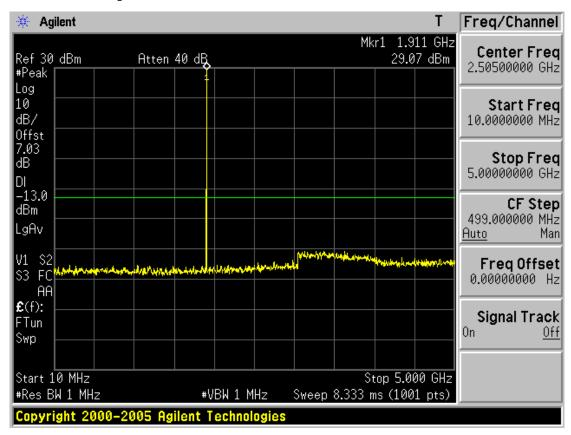
Spurious Emissions at Antenna Terminal / Ch.810 -1
