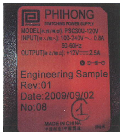
Power supply marking plate
