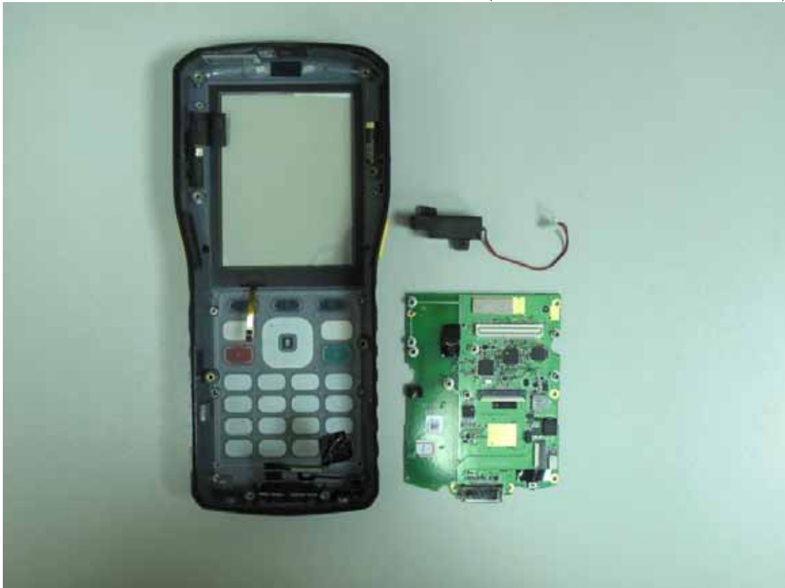
Figure 47 Internal View (Removed Button Control Board)
