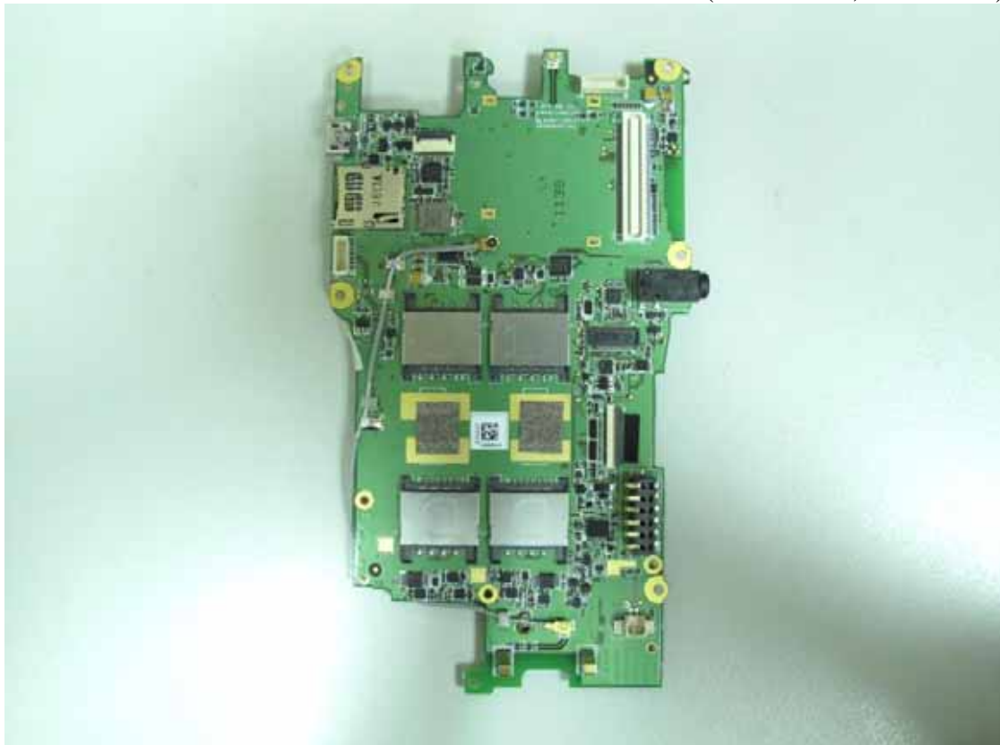
Figure 30 Internal View (Main Board, Front View)
