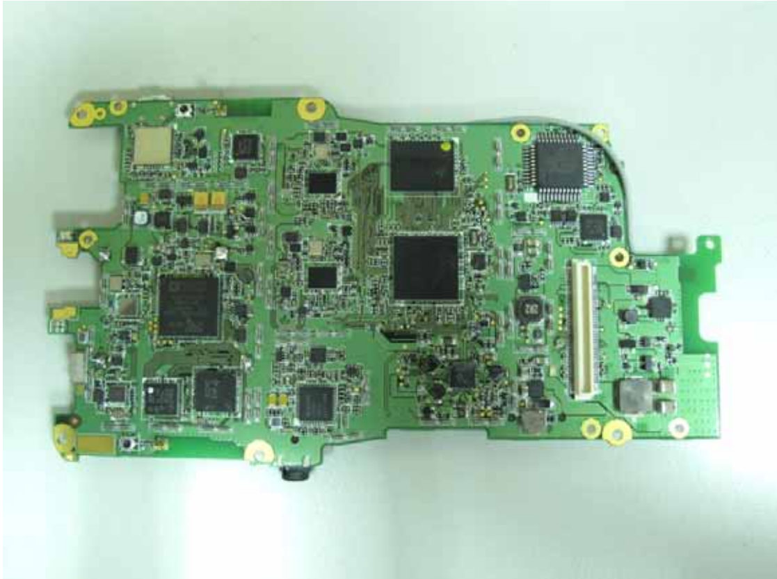
Figure 33 Internal View (Main Board, Back View and Removed LCD Panel)
