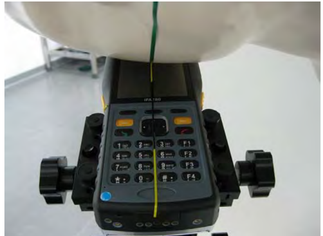
Fig.4 Right Head Section / Ear-Tilt Position(15°)
