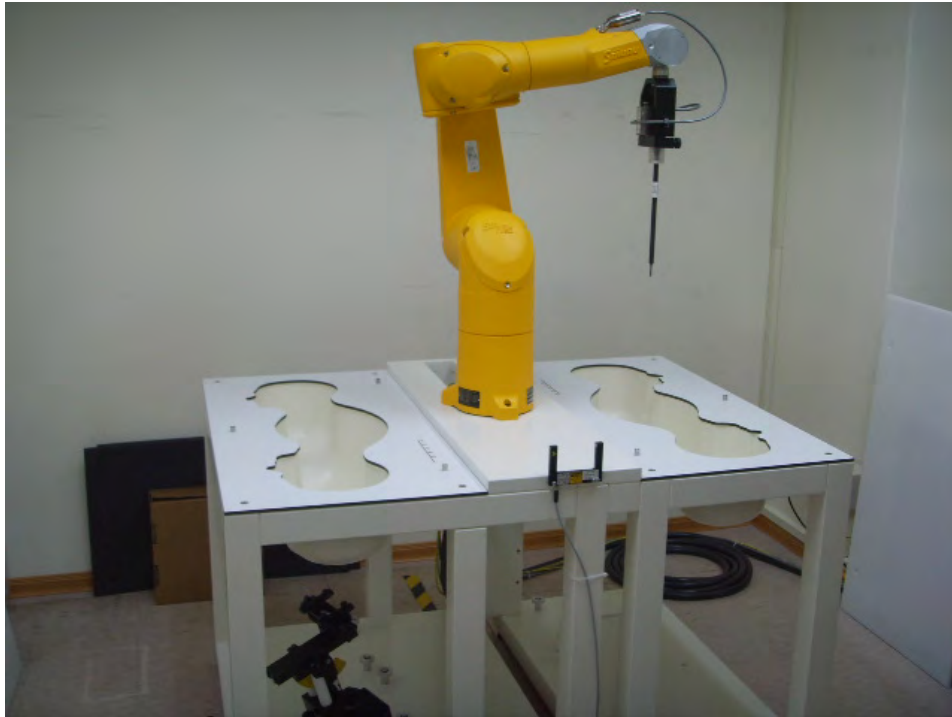
Fig.1 Photograph of the SAR measurement System
