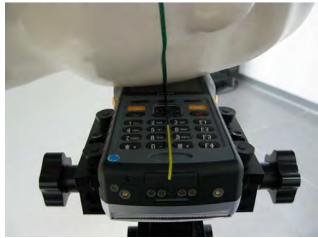
Fig.5 Left Head Section / Cheek-Touch Position
