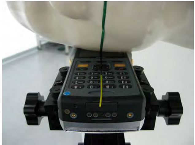
Fig.3 Right Head Section / Cheek-Touch Position
