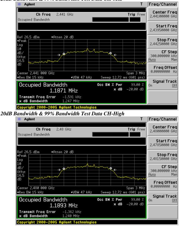
20dB Bandwidth & 99% Bandwidth Test Data CH-Mid
