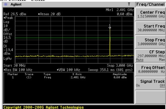
Conducted Spurious Emission Measurement Result (BDR mode) Ch Low 30MHz – 3GHz
