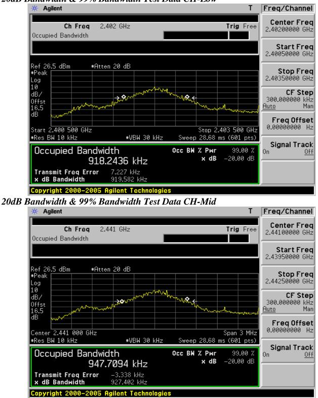
**BDR** Mode 20dB Bandwidth & 99% Bandwidth Test Data CH-Low
