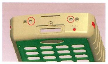
Add two Golden Pin onto the bottom of PDA for charging by upcoming design of PoGo Pin contact on new cradle & Car Kit.
