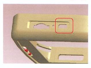
A DC jack is created just next to current Micro SD slot for charging by 5V/2A PSU.
