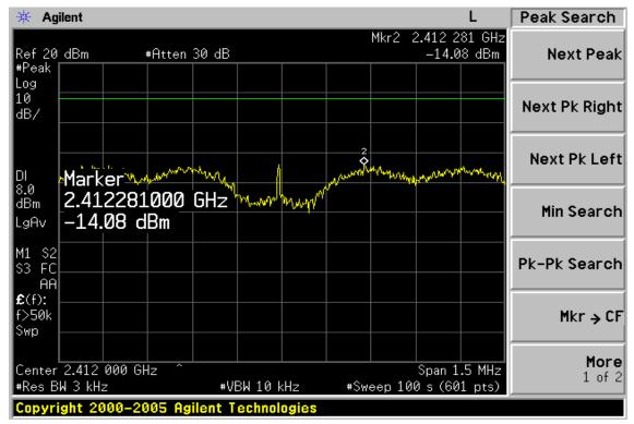
**Power Spectral Density Test Plot (CH-Mid)**
