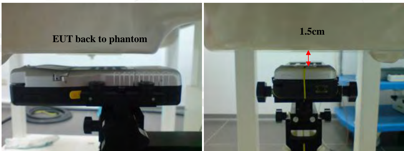
Fig.8 Body worn- EUT back to flat phantom and distance between flat phantom and mobile phone is 1.5 cm
