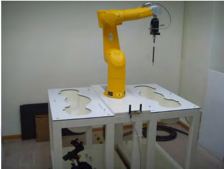
Fig.1 Photograph of the SAR measurement System
