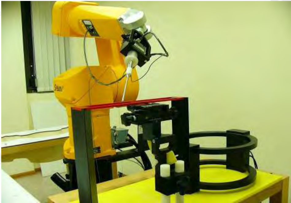
Fig.1 Photograph of the DASY 4 measurement System
