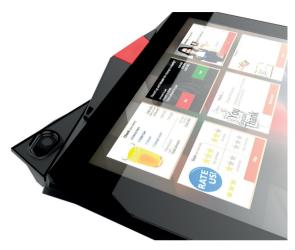
The Lane/8000 can be equiped with a module integrating a 5 megapixels autofocus camera.
