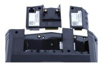
Insert the SAM Card into the slot marked (1), (2) or (3). Take care to ensure that the SAM Card is inserted in the correct manner. The cut corner must be positioned as indicated on the figure helow
