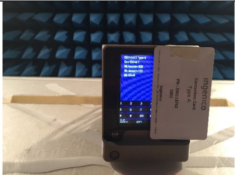
Axis Z above 1GHz in anechoic chamber
