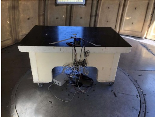
Test setup on OATS(30MHz-1GHz)
