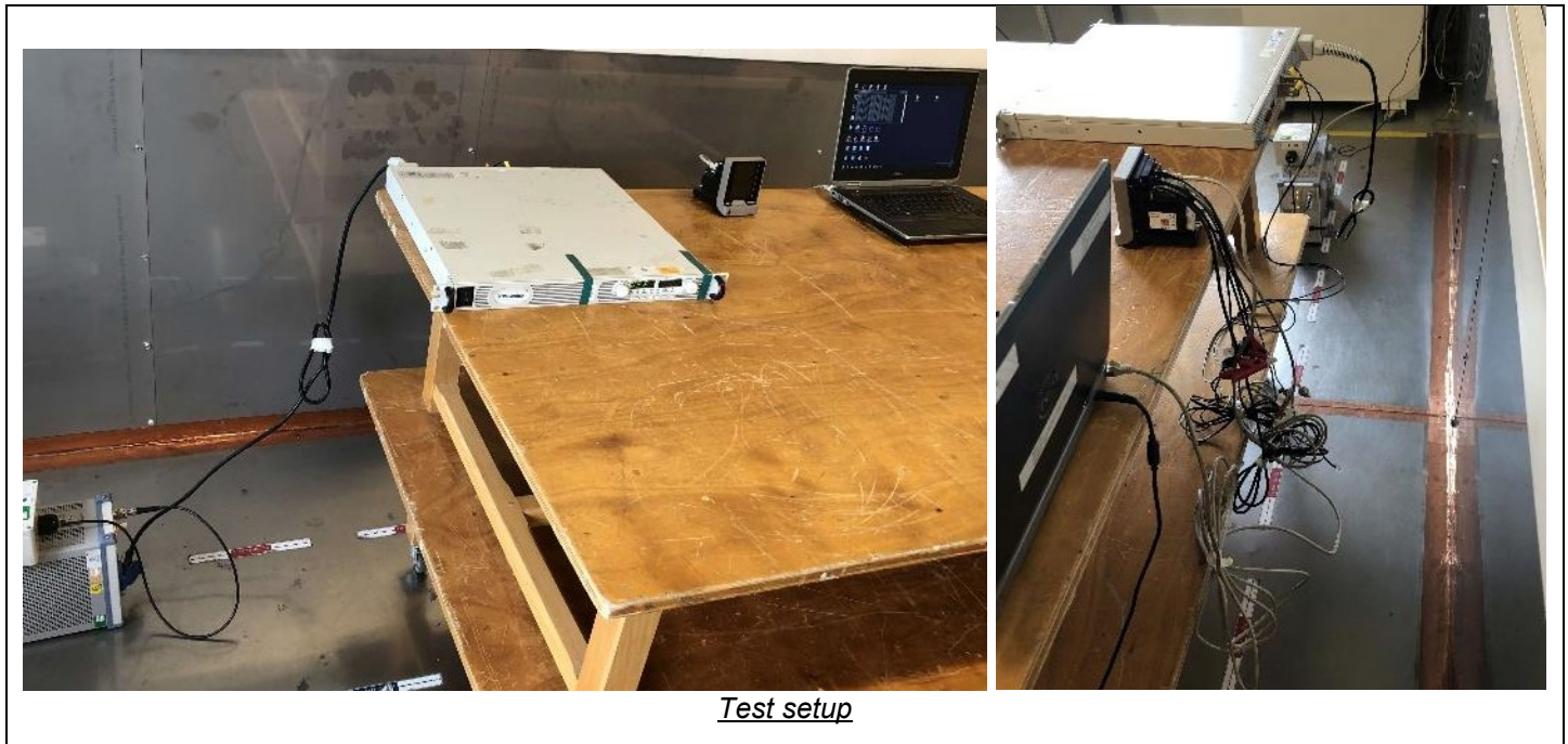
Photograph for AC Power Line Conducted Emissions (Front view)
