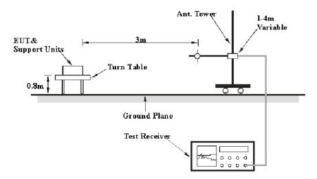
The radiated emission tests were performed in the 3-meter chamber test site, using the setup accordance with the ANSI C63.10-2013.
