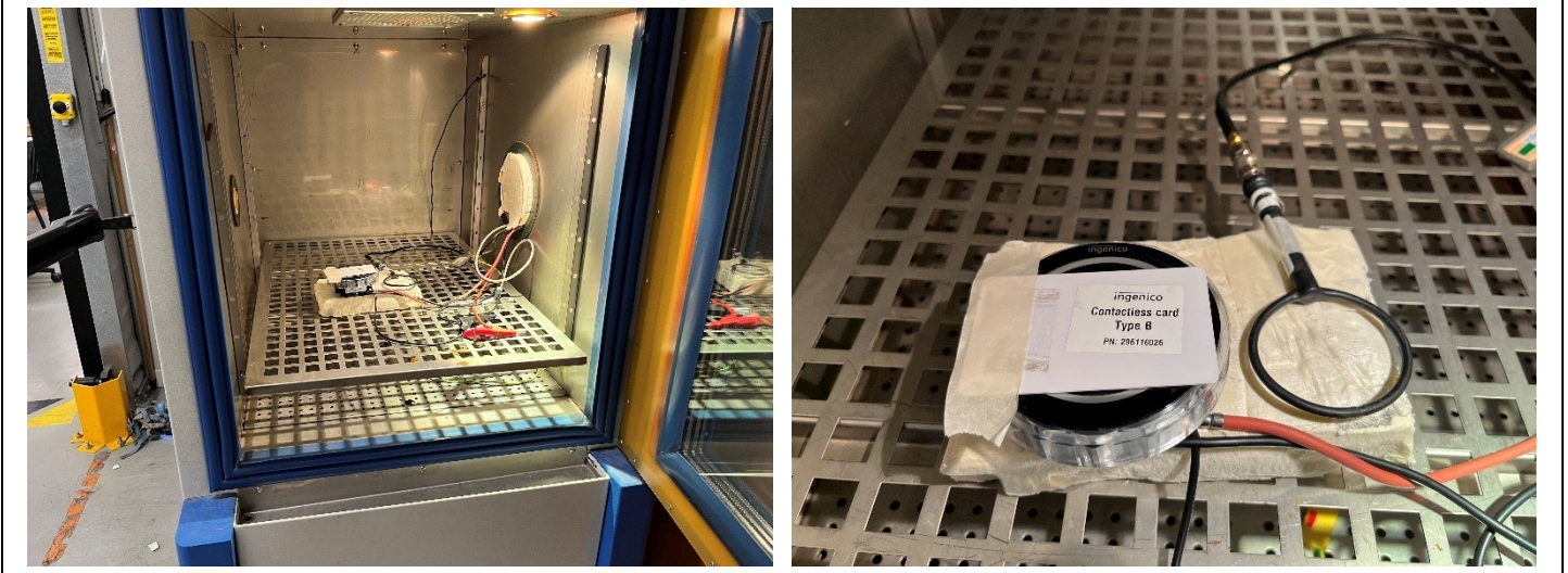
Photograph for Field strength within the band 13.110-14.010MHz in Climatic Chamber (normal condition)
