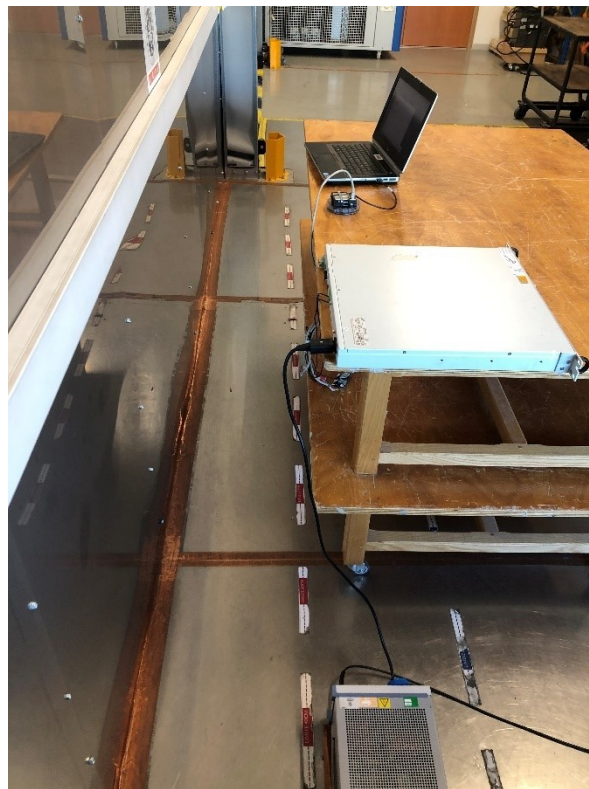
Photograph for AC Power Line Conducted Emissions
