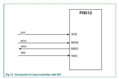
The PN512 acts as a slave during the SPI communication. The SPI clock SCK has to be generated by the master. Data communication from the master to the slave uses the Line MOSI. Line MISO is used to send data back from the PN512 to the master.
