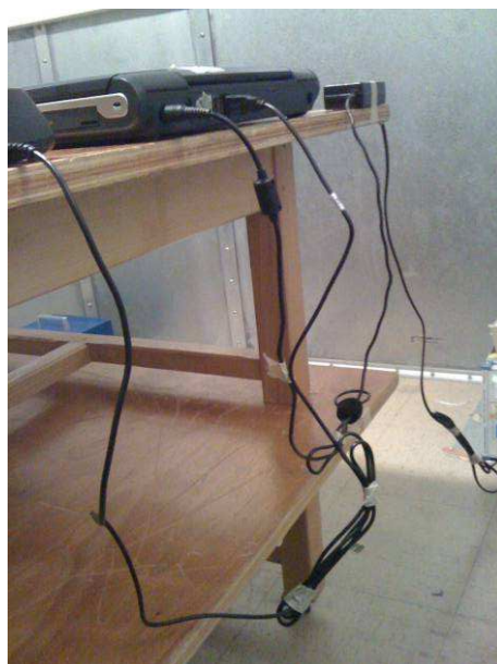
Radiated emission test setup – USB mode
