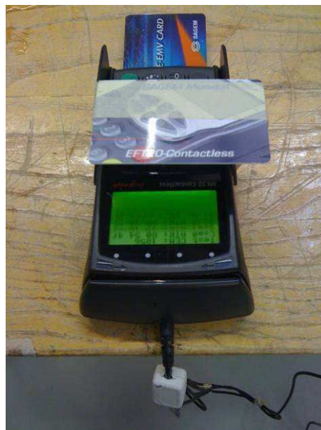
Radiated emission test setup – USB mode
