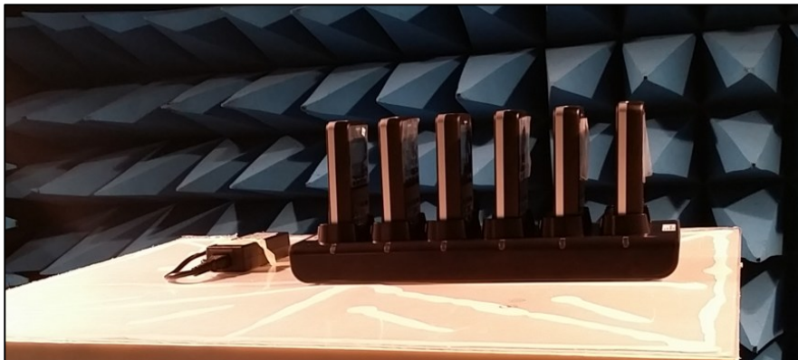
Test setup in anechoic chamber >1GHz
