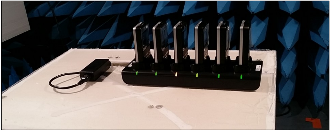
Test setup in anechoic chamber <1GHz
