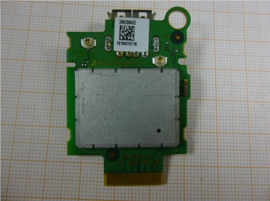
Photo 5: PCB front side view with shielding
