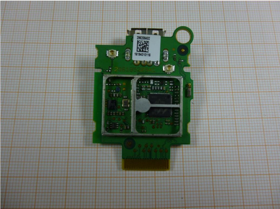
Photo 6: PCB front side view without shielding
